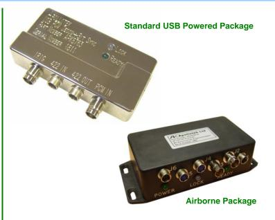
The Apollotek APK8763 Bit Synchroniser series are part of the ApolloDas range of USB products which are designed for PCM Flight Test Instrumentation system checkout and test applications. The Unit is incorporated into an aerospace grade aluminium housing machined from solid which is rugged enough to be installed in an aircraft.
